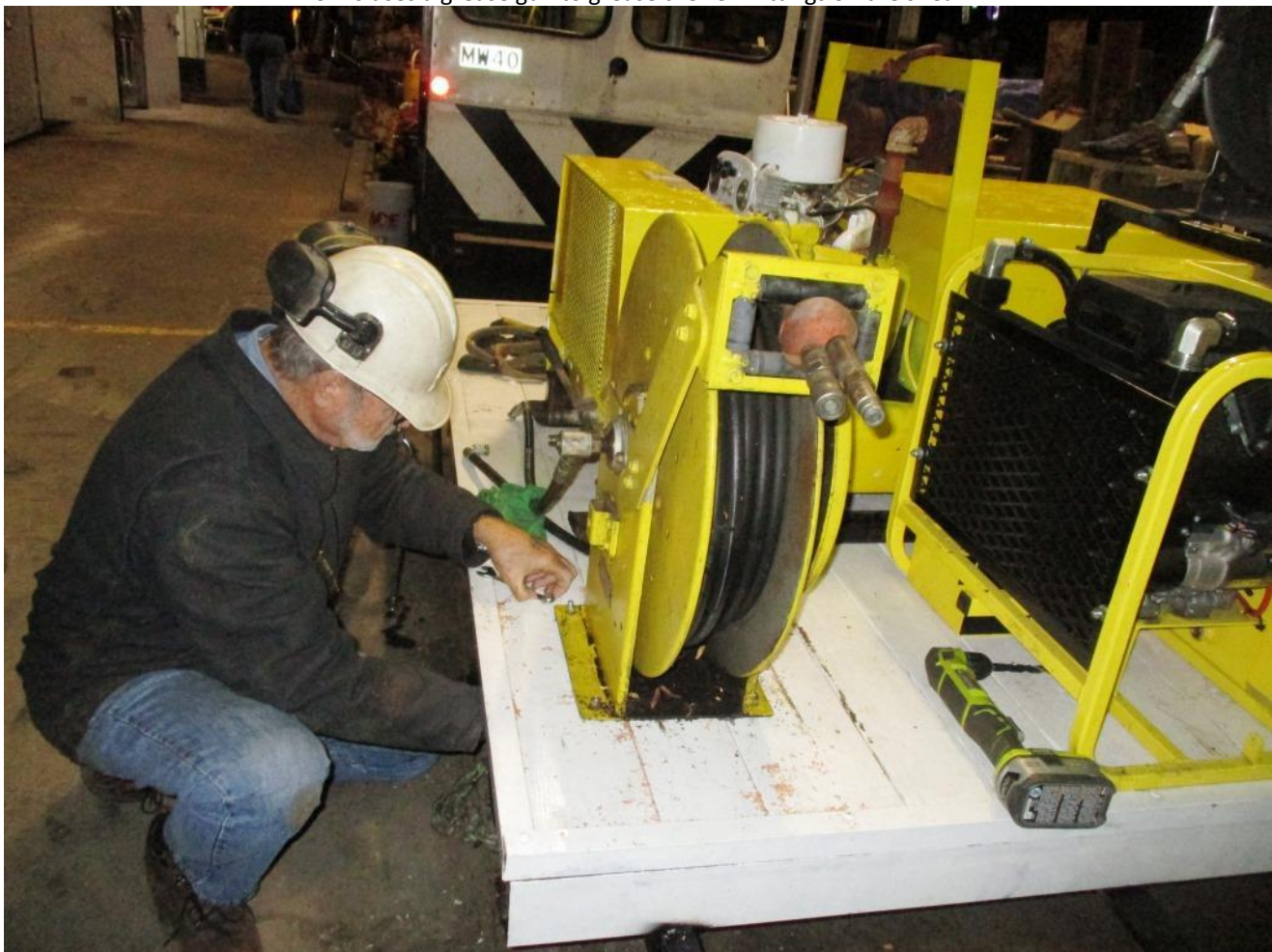
Alan bolts-down the hose reel on the new dedicated hydraulic power-units' flatcar that he has built
