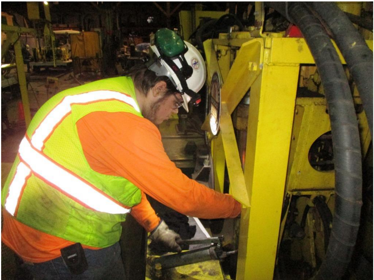
Chris uses a grease gun to grease the zerk fittings on the shear
