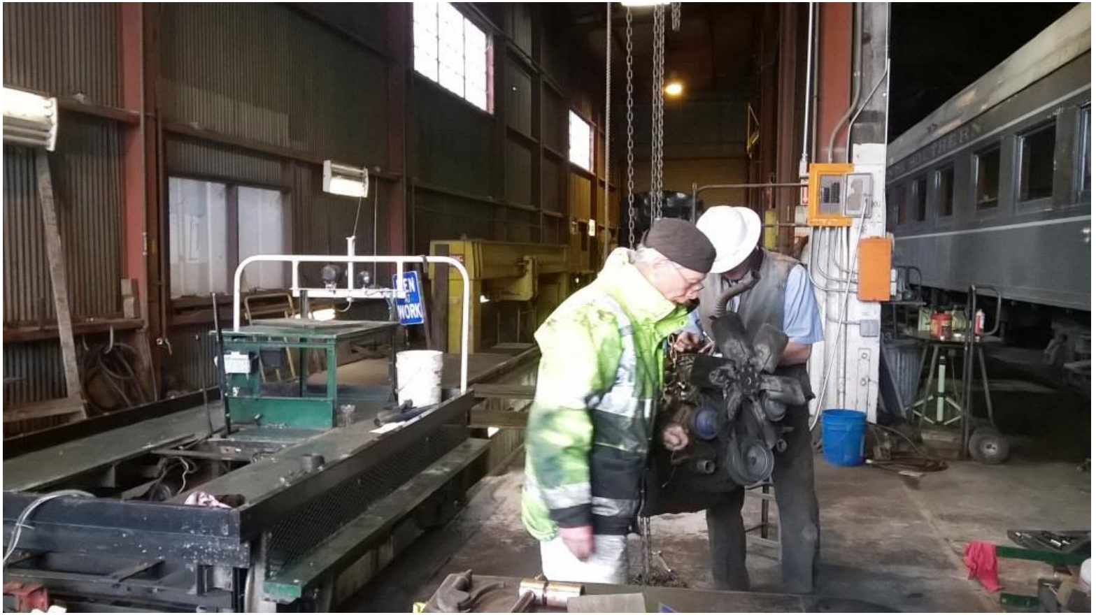
Jim Bays successfully removes the engine and transmission from the A-6 motorcar
