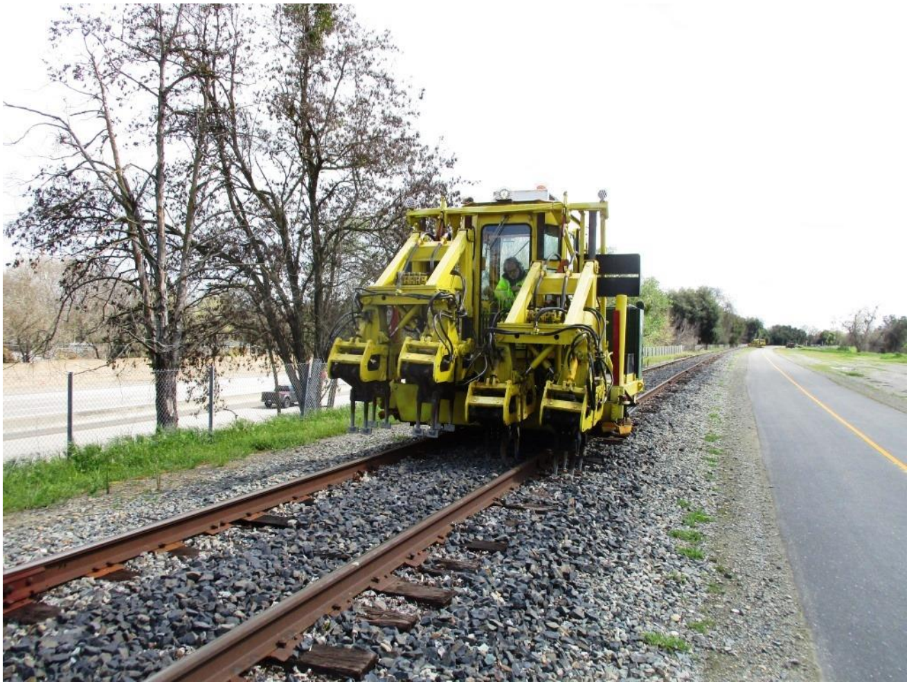
Further up the line, Alan tamps low joints near MP 2.4
