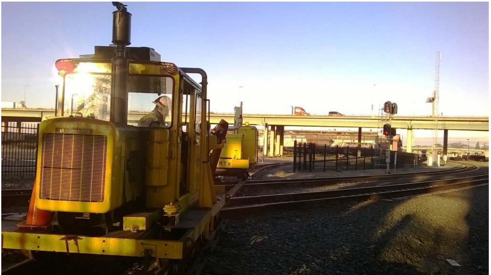
Because the tie-crane does not activate the signal system, the Kalamazoo, which does, traveled with it
